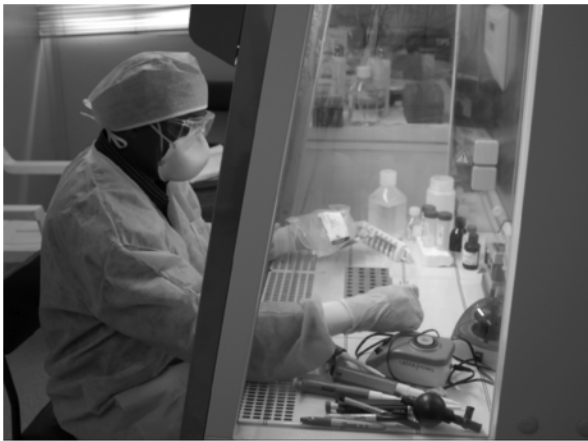
Fig A. Sample Processing in the Kenema Government Hospital Lassa Laboratory. Samples are manipulated in class II biosafety cabinets by personnel wearing full personnel protective materials.
