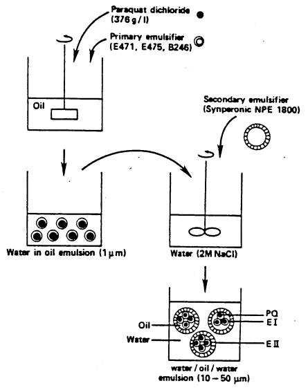
Multiple emulsion formulations of paraquat are based on containing paraquat within a water/oil/water emulsion. They are made by mixing a primary emulsifier with a paraquat concentrate in an oil. This mixture then undergoes a secondary mix with another emulsifier to produce droplets which are  $10\text{--}50\mu\text{m}$  in size. On dilution, the herbicide is released by osmotic disruption of the droplets.
